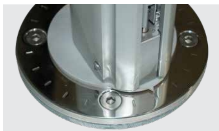
Figure F Align the indicator arrow with a notch
